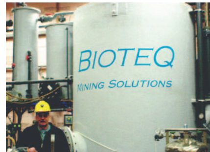
The Caribou operation provided a large-scale commercial demonstration of BioteQ's BioSulphide® process, using biologically generated H 2 S to recover dissolved metals from mine impacted water.
