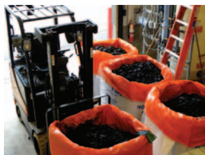
The high-grade metal sulphide recovered from the sulphate precipitation process can be recycled into useful products, eliminating the production of residual waste sludge.
